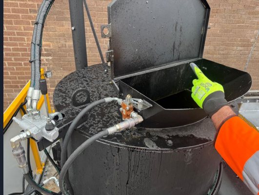
Lift the loading lid to empty any excess material from the buckets back into the mixer
