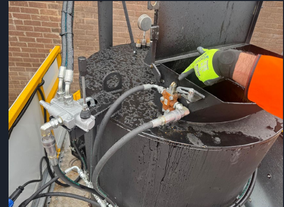
When opening the loading hopper, the paddles will stop spinning. When closing the loading hopper the paddles will re-engage
