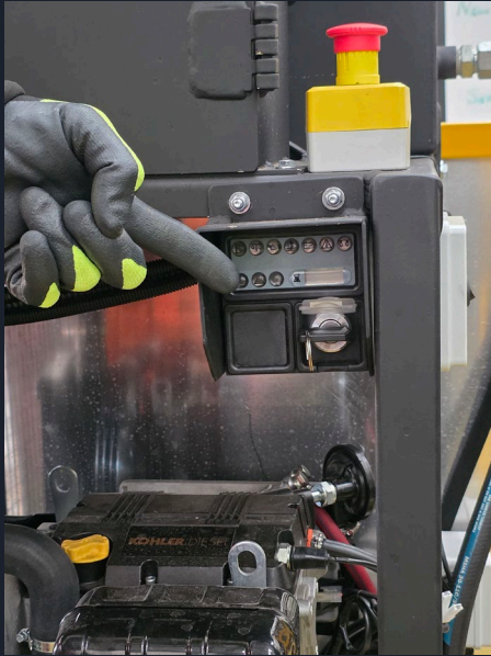
Turn on engine at keyswitch panel
